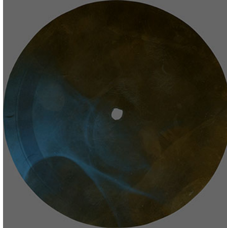
Pic. 2.1-4. One-sided flexible 6.4" (16.2 cm) record made of X-ray pattern (working side, carrying the sound groove, is shown) with the song All My Loving by The Beatles (the song's title and artists are not listed on the record). Rotation speed is 33 1/3 rpm.
