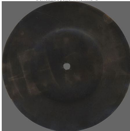
Pic. 2.1-2. One-sided flexible 6.0" (15.2 cm) record made of X-ray pattern (working side, carrying the sound groove, is shown) with the song Boys by The Beatles (the song's title and artists are not listed on the record). Most likely, rotation speed is 33 1/3 rpm.
