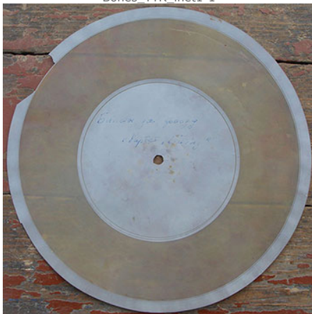
Fig. 1.1-1. One-sided flexible 8.9" (22.5 cm) record made of X-ray film (working side, carrying the sound groove, is shown) with the song Ticket To Ride by The Beatles (the song's title and artists are listed by hand in Russian translation – Билет за проезд, квартет „Битлз“ ). Rotation speed is 78 rpm.
